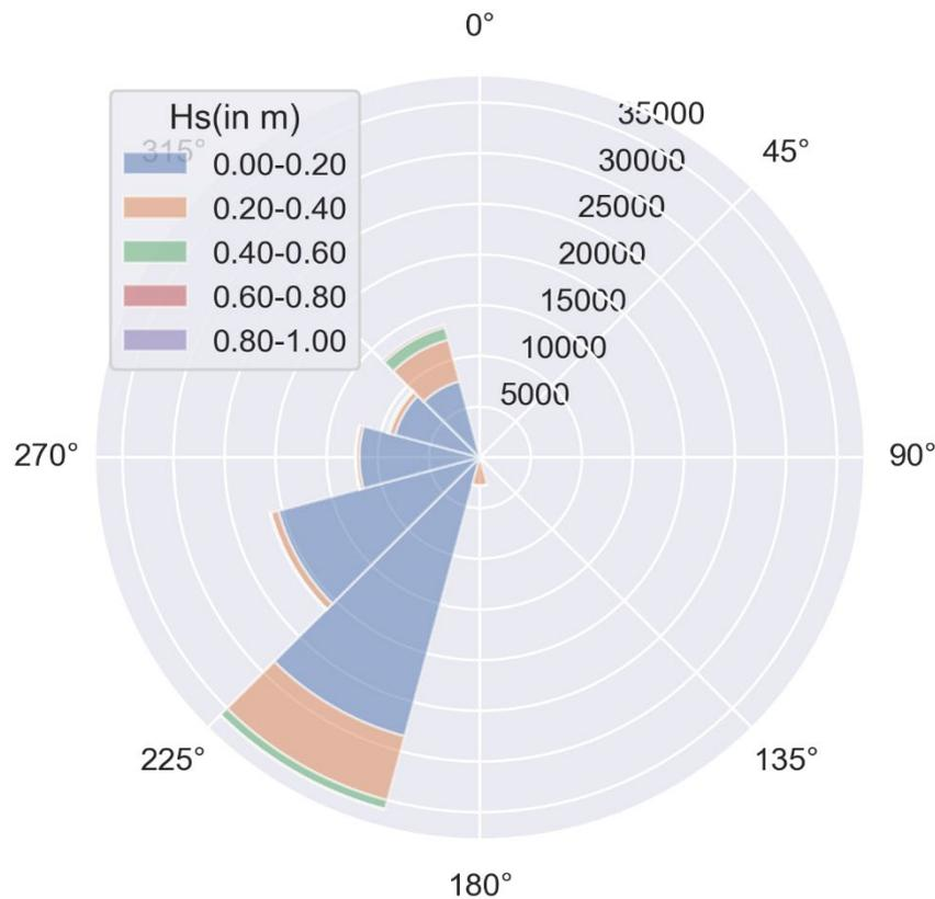
Figure 3. Wave rose for the planned ferry crossing, data for 2002-2017.
